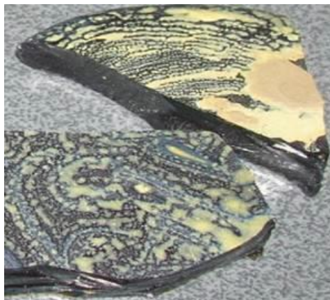
Example of a “yellow phase” due to a liquid-liquid phase separation coming from a high molybdenum content (courtesy of Dr. S. Schuller)
